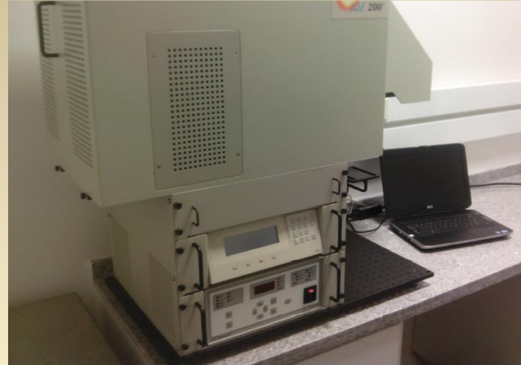
Sistema de medida de eficiencia cuántica QE- Oriel IQE-AC-QTH-SI-220. Software IQE 200 – Quantum Efficiency Measurement System v. 2.5
