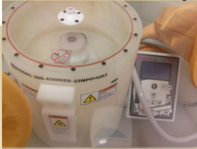
Spin Coater Laurell Technologies, WS-650Hz-23NPP-UD-3. Software Spin 3000
